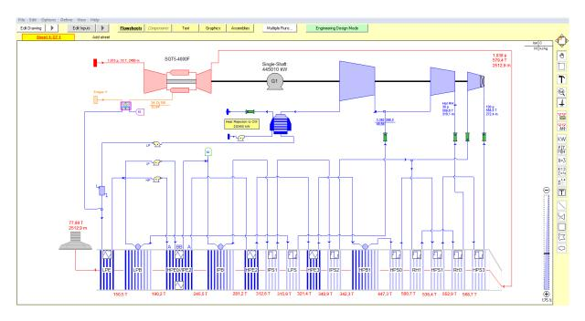
**THERMOFLEX** provides the **GT PRO®** gas turbine library and a reciprocating gas and diesel engine library which in the latest Version includes more than **700** gas turbine and **380** gas/diesel engine specifications. The **Steam Turbine Assembly** feature provides automatic estimation of efficiencies, leakage flows and information about the entire steam turbine such as dimensions, weight and costs.
